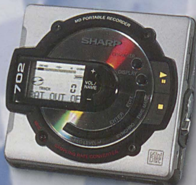
▶ Sharp and Sony introduce portable MiniDisc recorders. This digital alternative to audiocassettes records customized music compilations and doesn't skip when bumped.
