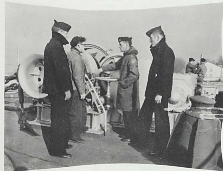
This is the anchor windlass— The wildcat—etc.
