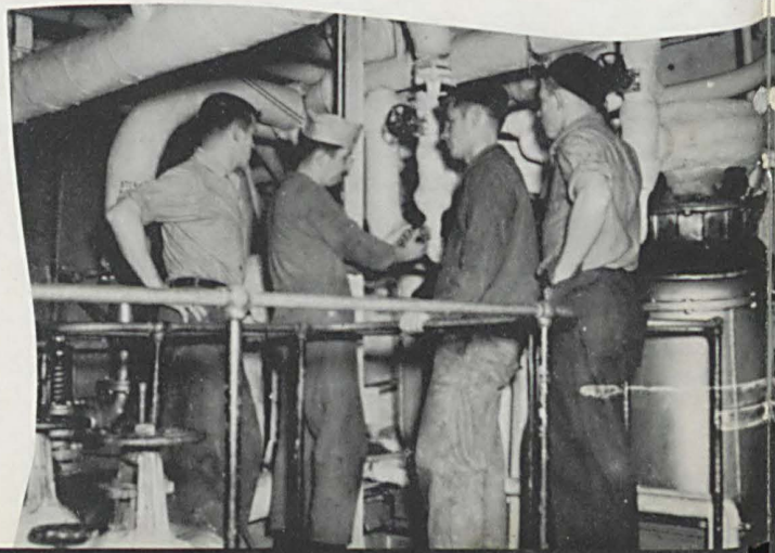
We all traced lines—Main Steam—Lube Oil—Here we are starting the Draft Fans.
