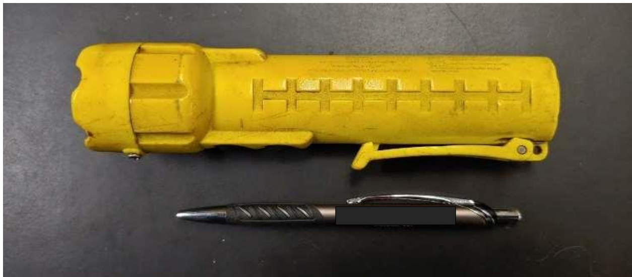
FLASHLIGHT: Practical size that fits in your pocket and bright/beamed enough to illuminate bilge recesses. Should be OSHA Approved and Explosion Proof.
