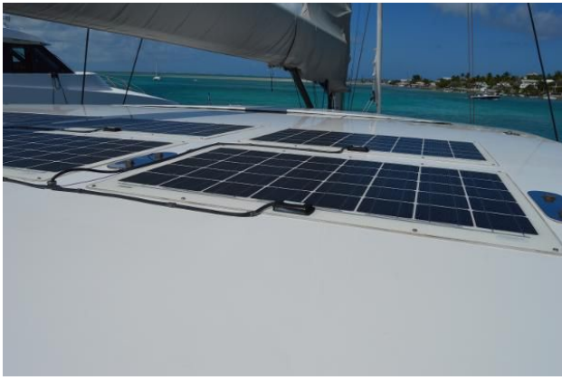
Solar Panels on Hardtop
