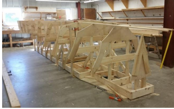
Figure 2.8: Construction jig for upper hull structure in place at The Landing School.
