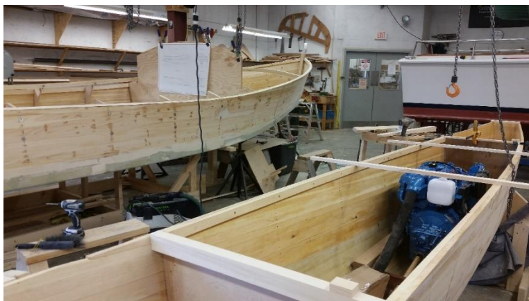
Figure 2.9: Construction progress showing diesel engine in main hull.
