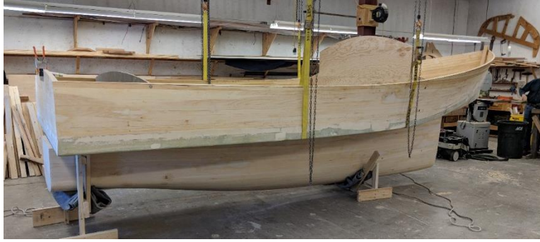
Figure 2.10: Test fit of upper hull to main hull. Note removable bow section.
