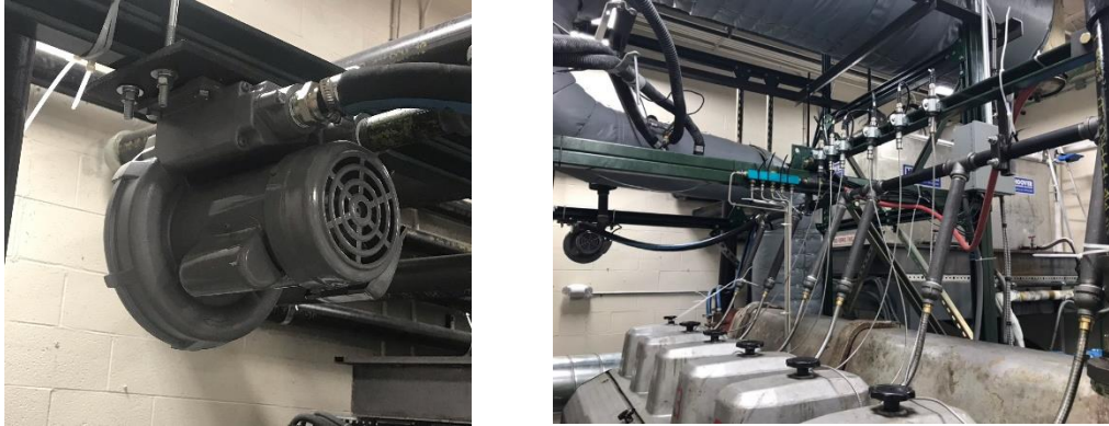
Figure 2: In-cylinder pressure sensor cooling system
