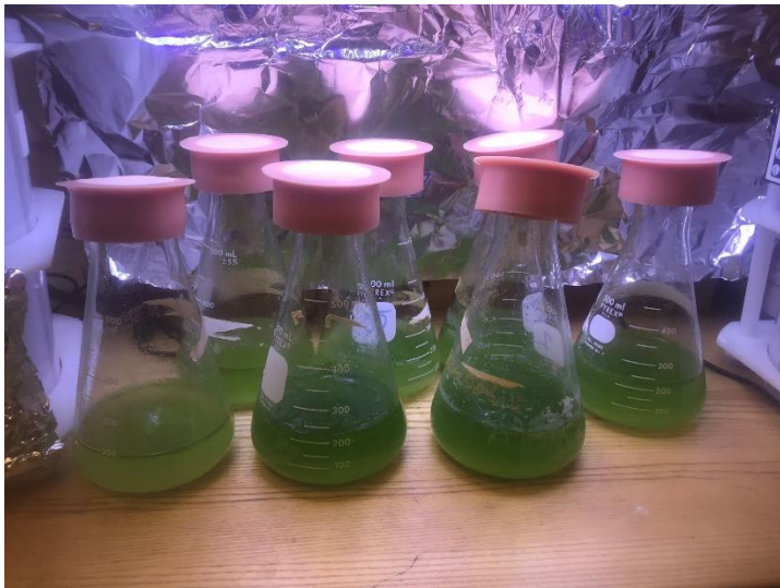
Figure 4: Algae Osmotic shocking experiment: Culture setup
