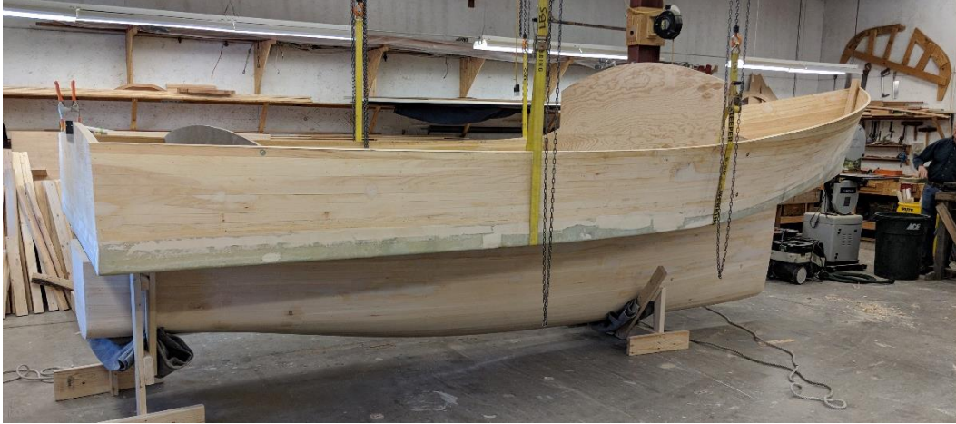
Figure 10: Test fit of upper hull to main hull. Note removable bow section.
