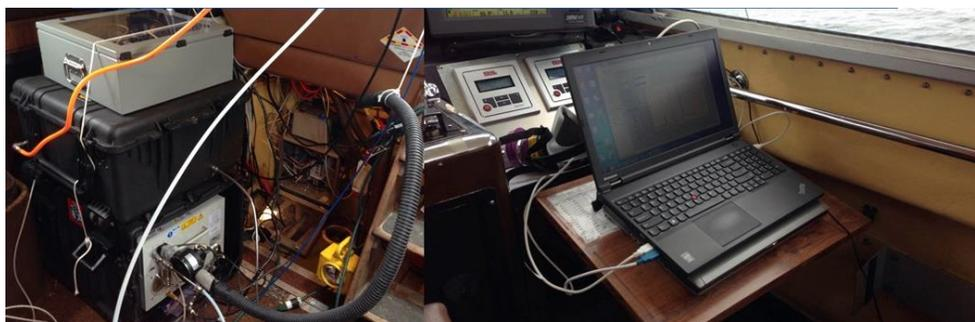
**Figure 3:** Photographs of floating engine emissions and data logging systems on-board the *R/V Quickwater* used during hydrogen injection performance testing.
