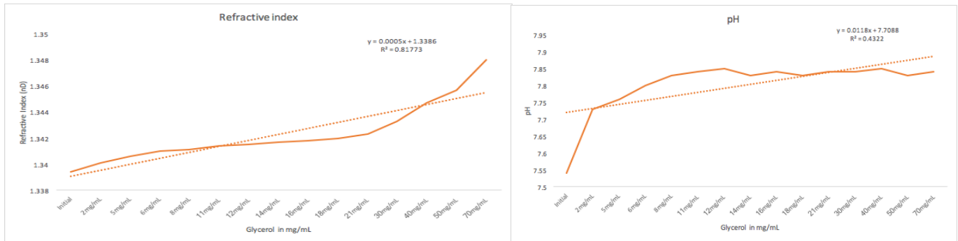
Figure 6. Measurements of refractive index & Ph to media samples with the addition of pure
