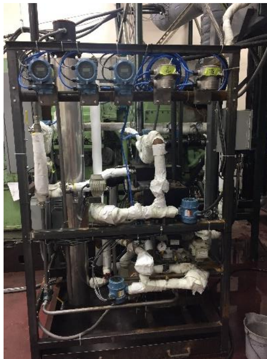
Figure 9: Photograph of fuel handling skid equipped with heat tracing, mass flow controller and viscosity monitors.
