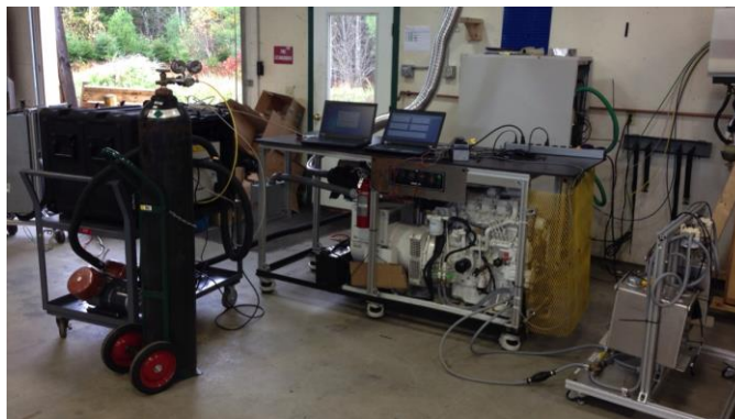
Figure 5.3: FTIR system and gaseous emissions test during engine warm up.
