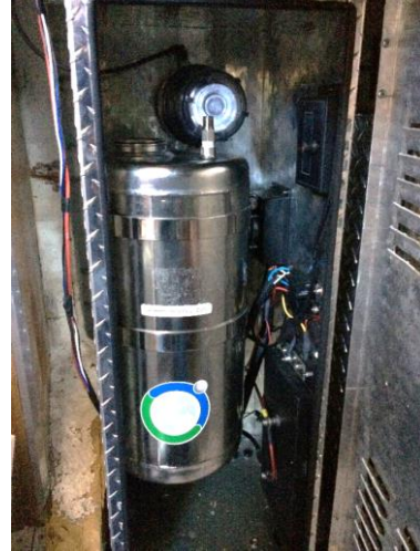
Figure 2.2: Hydrogen generation system on board Quickwater .
