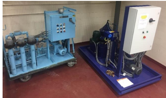
Figure 8: Oil and fuel purifiers, from left to right
