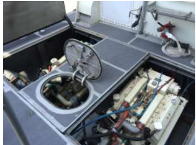
Figure 2: Twin Cummins diesels onboard Quickwater.
