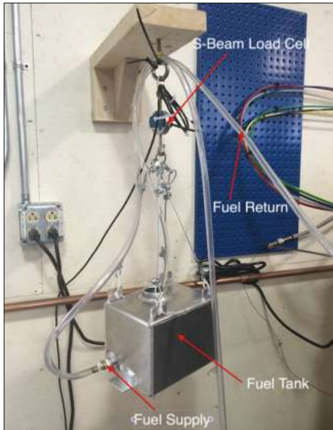
Figure 6: Fuel flow measurement system.
