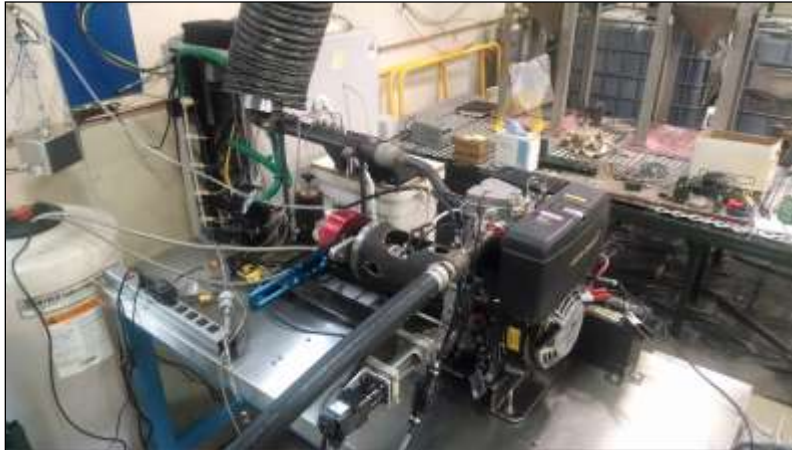
Figure 4: METEL Single Cylinder Diesel Engine Test Stand
