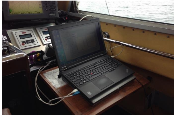
Figure 8 Computer running CEMS LabVIEW vi placed in the cabin aboard Quickwater during testing.
