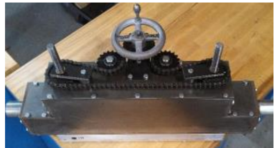
Figure 4: TEG Exhaust Test Apparatus
