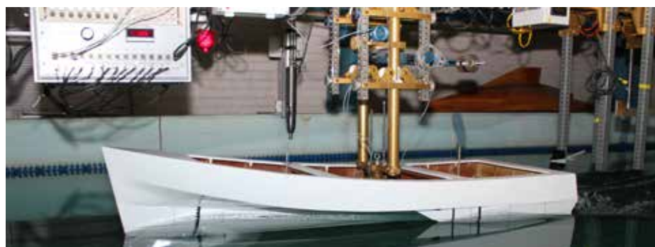
..... Scale model of trimaran lobster boat hull being tested, photo by D Read.
